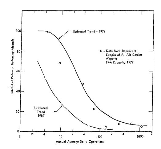
Figure A-5. Estimated Percent of Airport Operations Carried Out by Propeller Aircraft
