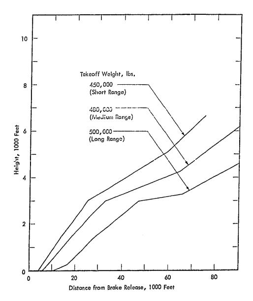
Figure B-5. Takeoff Profiles for Level III Technology, 3-Engine Aircraft
