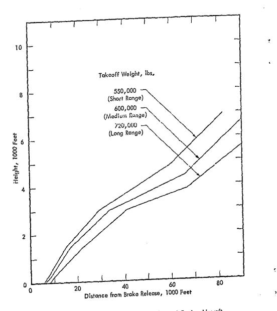
Figure B-6. Takeoff Profiles for Level III Technology, 4-Engine Aircraft
