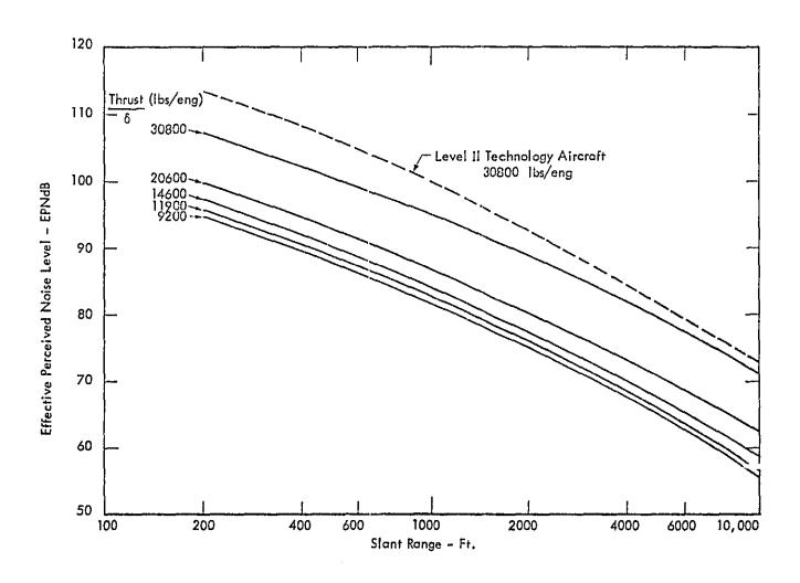
Figure B-1. Noise Curves for Level III Technology - 2 Engine Aircraft.
