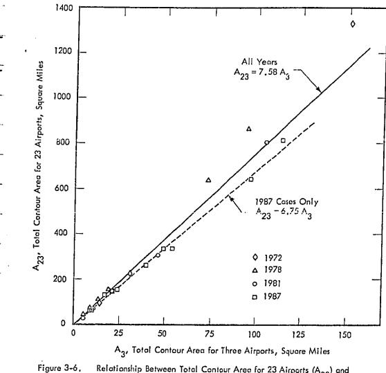
re 3-6. Relationship Between Total Contour Area for 23 Airports (A<sub>23</sub>) and Three Airports (A<sub>3</sub>). (For the sake of illustration these simple regression lines were forced through the origin.) Data from Reference 1 for all alternatives and NEF values.
