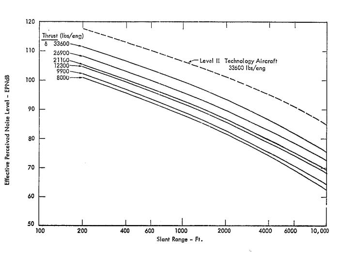
Figure B-3. Noise Curves for Level III Technology - 4 Engine Aircraft.
